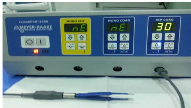
**Figure 1:** Bipolar Radiofrequency Ablation Device (Radiosurg 2200, ENT Version, 2.2 MHz, Meyer Haake, Germany,) with the small conventional reusable bipolar cautery forceps.
