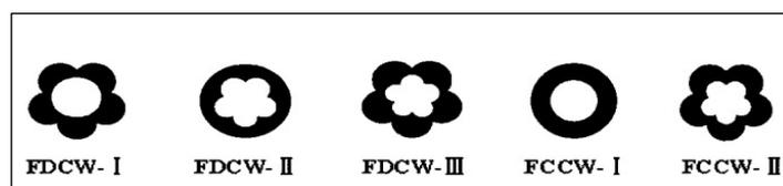
**Figure 1: Various types of cavities depending on internal and external wall characteristics**
