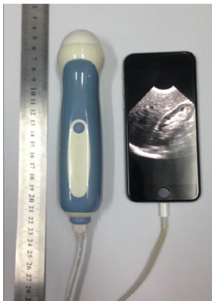
Figure 1: Ultrasonographic probe connected to smart phone.
